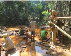
The above photos were taken on January 5<sup>th</sup> 2013 in Shwegyin Township, Nyaunglebin District. They show gold miners using a process known as cyanidation. This process involves placing crushed ore into piles where a cyanide solution is poured over it in order to allow the gold to 'leach' out of the pile. However, this process risks contaminating the surrounding area with cyanide and is heavily regulated by many nations. [Photos: KHRG]
